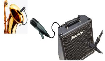
If you have a microphone on something, and you want a bigger sound, you could place a second microphone at the source and then connect that to a Loudspeaker Cabinet where you place a microphone. Now you have two sound sources for the same instrument, but with very different sound material.
